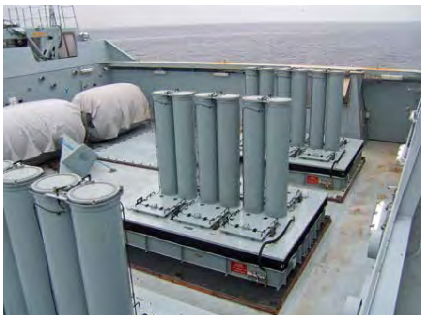
An example of a Standard Flex module: A Mk 56 vertical launcher module pictured here installed amidships on the Royal Danish Navy's ABSALON.
