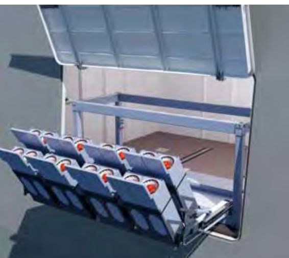
An Unmanned Aerial Vehicle (UAV) side launch container conceptualised by SH Defence as part of The Cube
