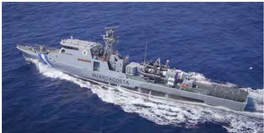
This OPV supplied to Honduras was based on the combat-proven SAAR 4.5 hull form.
